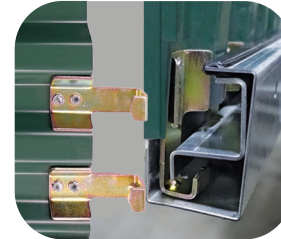
As wind blows against the 988WL, the curtain's windlocks engage with the door guide for a strong interlocking grip. This grip keeps the curtain securely in the guide.
