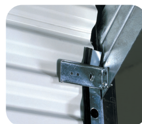
12-gauge, zinc-coated door stops are mounted to brackets for increased strength. 18-gauge, zinc-coated steel guides with polypropylene runners allow doors to glide smoothly.
