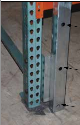
Select a mount height to line up with two of the three holes.
