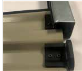
As wind blows against the 977WL, the curtain's windlocks engage with the door guide for a strong interlocking grip. This grip keeps the curtain securely in the guide.
